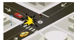
Intersection collision warning
